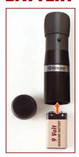
**Battery Insertion:** Remove the battery end cap from the unit and insert the 9V Lithium battery into the barrel. The polarity of the battery is interchangeable; the + or - battery poles are reversible. Electrical contact will be made automatically when the barrel end cap is screwed onto the end of the barrel
